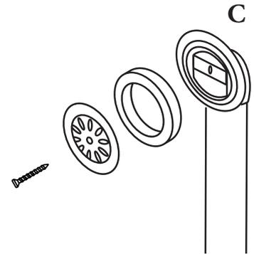
**5** Trim drain pipes. Connect the overflow and drain assemblies and pipes to the tub.
