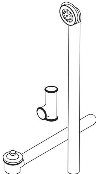
**6** Attach the waste and overflow tee (D) to the overflow assembly (C) and shoe assembly (A) with sealing washers and slip nuts.
