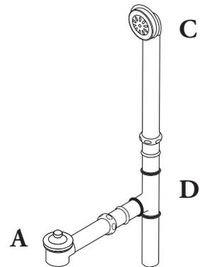
**7** Attach the drain tube and flange (E) to the waste and overflow tee (D) with the sealing washer and slip nut.
