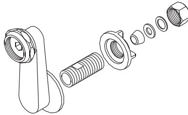
3. Attach the diverter lever (C) onto the diverter valve (D) and tighten the diverter screw.
