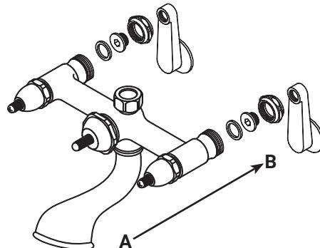
2. Thread the tapered ends of the nipples into the swivel mounts on the outside of the tub.
