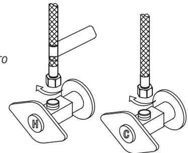
**IMPORTANT: The hot side inlet tube is indicated by a label. Avoid twisting wires together or placing the wires close to each other and damaging.**
