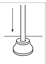
Attach the upper end of one supply tube to the "cold side", faucet connection tube located under the rim of your tub by inserting the supply tube into the faucet connection and tightly screwing the decorative locknut over the two for a tight fit.
