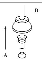
Attach the bottom end of each supply tube to the water supply in your floor by screwing the brass locknutdown tightly. Let the escutcheons slide down to the floor.
