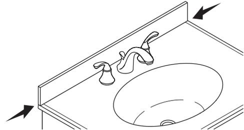
*USE SILICONIZED ACRYLIC CAULK TO SECURE TO THE WALL*
