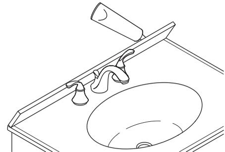
*FINISH BY APPLYING A BEAD OF CAULK ALONG THE SEAM OF THE WALL AND THE VANITY TOP.*
